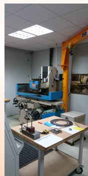
700x320 grinding machine and its 250kg crane
