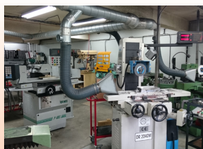
Grinding workshop with a centralised dust extraction system.
