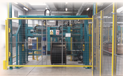
Unwinder with vertical sliding door
