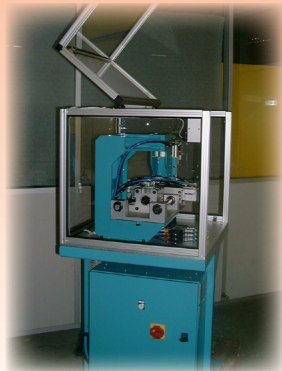
Individual stripper for cables from 10 to 95mm 2
