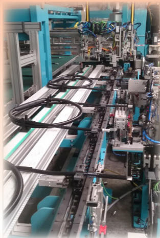
Individual stripper for cables from 10 to 95mm 2
