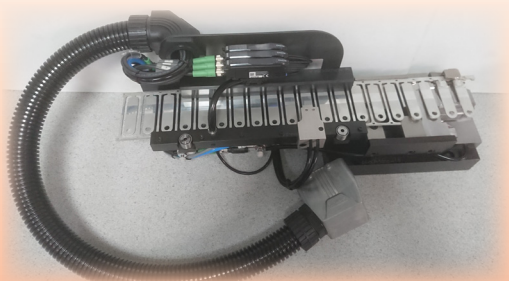
Lower cassette with sensor and band feed
